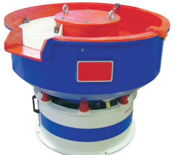
Vibratory bowl finishing machine
